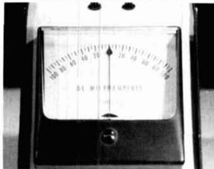
Zero center meter movement.
